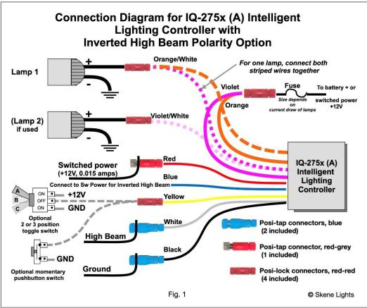
If several brightness settings are required, connect the yellow wire to a 2 or 3 position toggle switch or momentary pushbutton switch wired as shown in Figures 1, 3 and 4.
